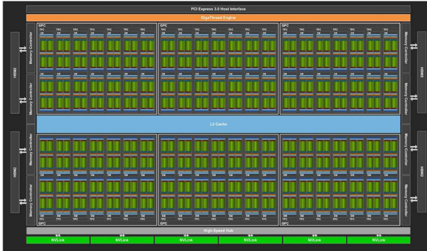
Figure 4. Volta GV100 Full GPU with 84 SM Units
